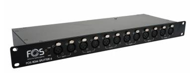
RDM 6 channel isolated Dmx splitter, Fully compliant to DMX-512 100% electrical isolation between in/output, Signal & power LED indicator, Terminator resistor switch, 3pin & 5pin input / through.
