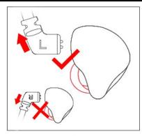
The correct assembly of the wire is with the needle head and "L R" logo facing up. Do not assemble the pin head down and it will have an adverse effect on sound quality.
