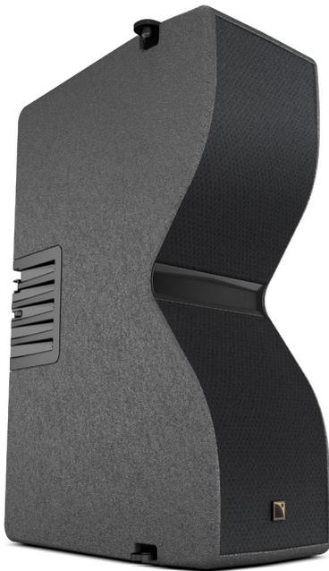
The Kiva II is an ultra-compact WST® modular line source designed for long-throw sound reinforcement applications with minimum visual impact. The Kiva II features two 6.5" speakers in a bass-reflex cabinet and a 1.75" diaphragm compression driver loaded by a DOSC waveguide and L-Fins.
