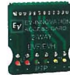
EVI-AC EV-Innovation Access Card lets you test EVA, EVF, or EVH transducers and protection circuitry without disassembling the cabinet.
