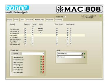
The MAC808 has the options to page separate outputs and combine independent outputs to a single zone.
