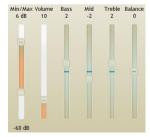
Like the default input also the default volume level, sound colour and balance can be set for each output. These are the default start up values after a power cycle or system standby. The balance option is only available for stereo outputs.
