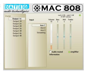
Tone adjustment can be done in the same easy way as volume control. Select the preferred level and it will instantly change to the new value. These changes are not permanent. On a system restart the configuration default values are loaded.
