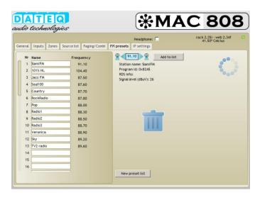
The MAC808 can store up to 50 tuner presets. These presets are used for all four tuners. Adding, removing or editing the names and frequencies can be done in the FM preset tab.
