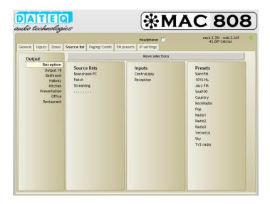
For each output a list of user selectable audio sources can be made. Each output uses it's own list.
