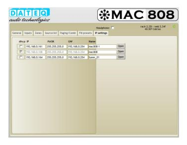
By default the MAC808 is set to DHCP\*. In a regular DHCP network that supports DNS\*\* the MAC808 can be reached through:
