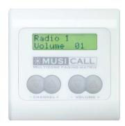
The wall units are mounted in each room (zone) and can be connected using a two wire cable to the MAC808. The MRC3 wall unit fits inside a standard electric mounting box and the MRC4 can be mounted directly onto a wall without the use of mounting boxes.
