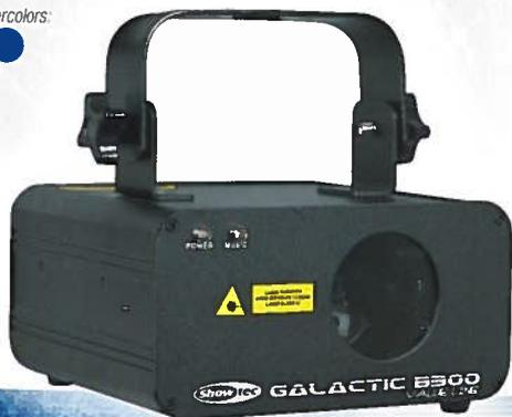
The B300 is the single blue color laser of the Galactic Value Line. It is equipped with a 300mW 450nm laser-diode. Just like the G40 it has 8 DMX channels and a total of 32 different patterns.
