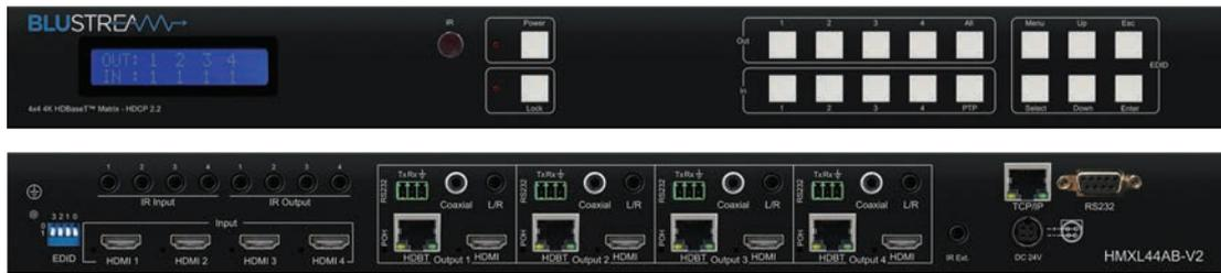
The HMXL44-KIT-V2 is a 4K HDCP 2.2 compliant 4x4 matrix package, delivering HDMI, Bi-directional IR and PoC up to lengths of 70m over a single CAT cable. The matrix also provides advanced features including audio breakout with pre-amp variable line-level control, simultaneous HDBaseT™ / HDMI outputs, RS-232 pass through to enable 3rd party control of displays and web interface module for control and configuration of the matrix. The HMXL44-KIT-V2 is supplied with 4 x HEX70ED receivers.
