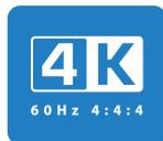
The 4K data rate varies depending on the requirement for varying frame rates, colour depths, and colour gamuts. 4K60 4:4:4 requires the full 18Gbps data transfer speed required to get the very best 4K image across your system.
