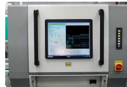
State-of-the-art Auto Optical Inspection System that zooms in on every solder joint
