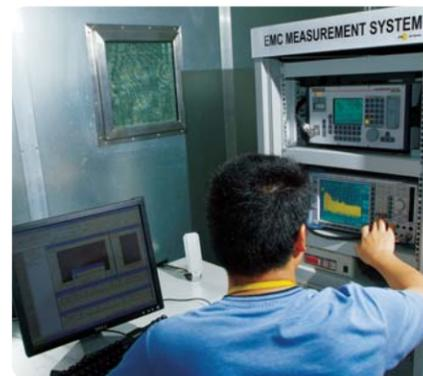
This is the Electromagnetic chamber where we test all products for compliance with standards such as FCC emissions, CE and safety. The facility represents a multi-million dollar investment and includes at least one machine that goes "ping"
