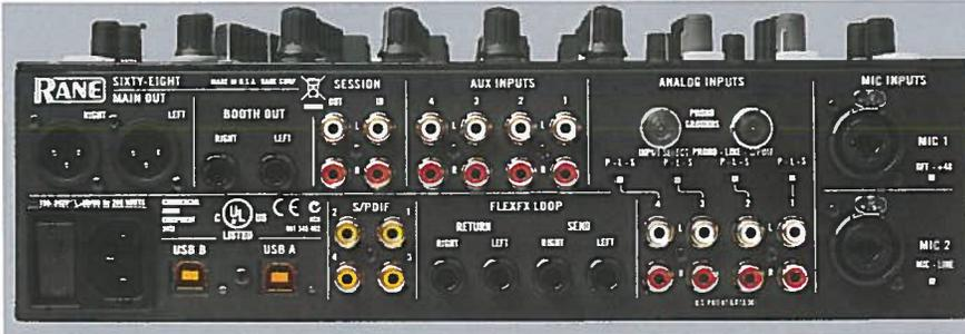
Using two USB ports, the Sixty-Eight lets two DJs use their laptops at the same time, allowing seamless handover between DJs. You can also control up to four decks with a single laptop.
