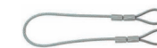
ESL 16 Câble acier galvanisé recouverte de polythène transparent 1500 mm x 8 mm – charge max. 1000 kg Steel sling covered with transparent polythene Wire 8mm Length 1500 mm.
