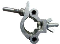
CUP 20 Collier aluminium pour tube ø 20 mm – charge max. 10 kg Aluminium Coupler for tube ø 20 mm – max load. 10 kg
