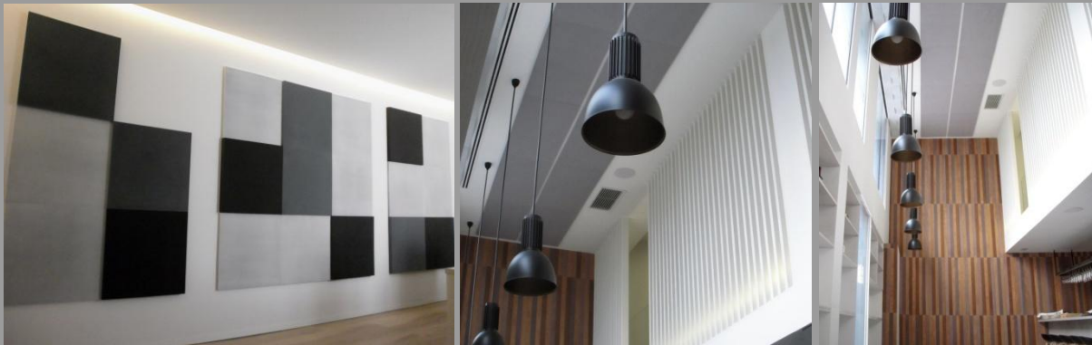
REGULAR PANEL 60.2 and 60.4 Premiere Dark Grey/Black/White on walls and Light Grey on ceiling.
