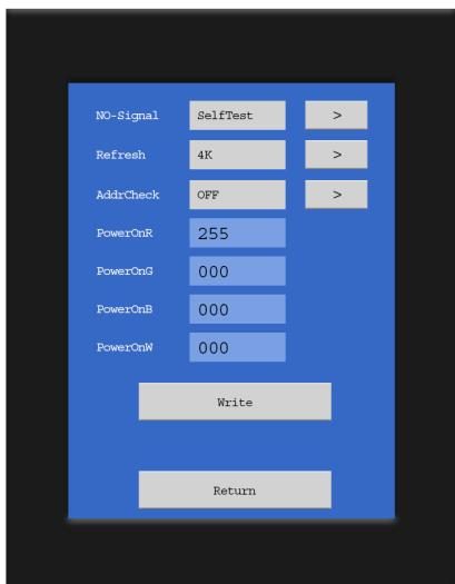
6. With the 'No-Signal' setting, configure the behavior when no DMX signal is detected. You can set this to:
