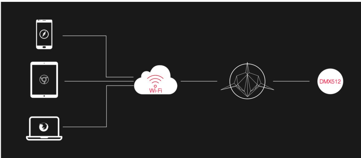
The LightShark software is always running inside the console (LS-Core or LS-1), in the WiFi connection between your device and the console only travels user interface data, never DMX data.
