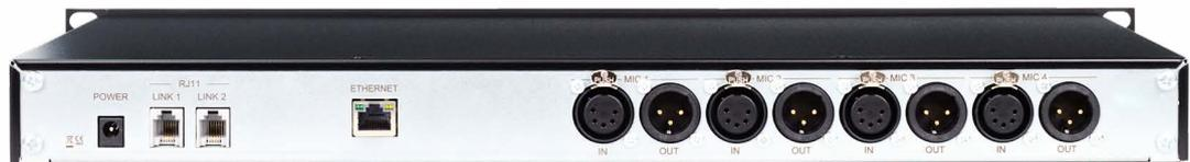
Up to 4 microphone arms can be connected to the rear panel of the MOS Quatro IP. The MOS Quatro IP will control the lights of the connected arms in red for on-air and white for off-air. The audio signal is routed directly from the connected microphone arm to a standard 3-pin XLR connector.
