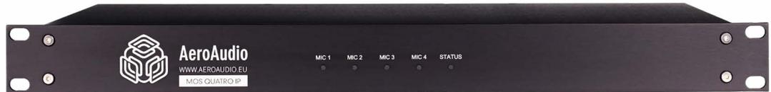
The indication LED's on the front panel of the MOS Quatro IP shows the status of each microphone. These LED's indicates whether the microphone arms are on standby, fixed white light, or fading in and out.
