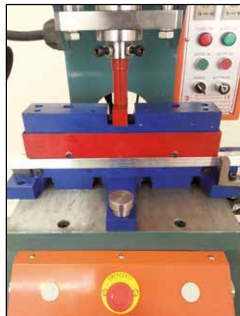
Stanzan von Löchern in Profile. Punching rivet holes in Extrusions.
