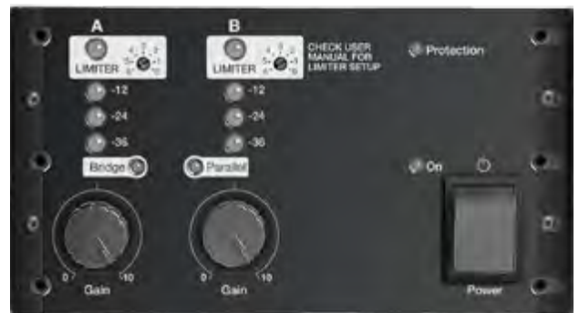
Detachable front panel gives access to a limiter threshold adjust. (LIMITER)
