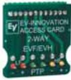
EV-Innovation Access Card lets you test EVA, EVF, or EVH transducers and protection circuitry without disassembling the cabinet.
