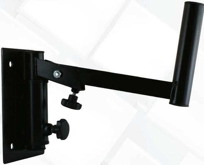
The SWB40 is a heavy duty wall mount bracket for loads up to 40 kg. It is slewable for 180° and tiltable from 90° to 110° downwards. The complete system is from black powder coated 2 mm steel.
